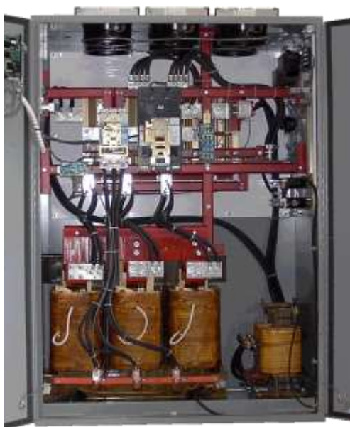
12 pulse large charger designed to reduce THDi & ripple
